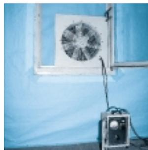
In the air test a special fan is used to produce a reduced pressure of 50 Pa (5 kP/m<sup>2</sup>). Air flows through leak points from the outside to the inside and is detectable as air pressure or visible using smoke tubes. The leak points can be sealed during the test.
