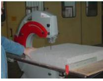
The maximal cut height is 160mm, the maximum projection 380mm. Mitre cuts up to 45° are possible by adjusting the angle of the cutting table.
