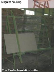
The Pieske cutting aid is suitable for simple straight cuts. Mitre cuts are not possible.
