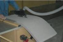
Cutting with stationary circular saw is particularly suited prefabrication work.
