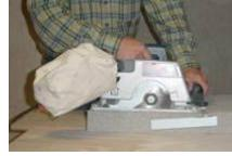
dust bag or extractor outlet next the hand-held circular saw necessary in order prevent unnecessary build up of dust particles.
