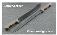
Whereas the serrated slicer is useful for cutting any cellulose batt, the Granton-edge slicer was specifically developed for use Homatherm on flexCL.
