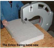
Cutting Homatherm with a band saw produces very clean edges with minimal dust creation.
