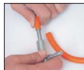
Cutting/Calibrating of pipes
